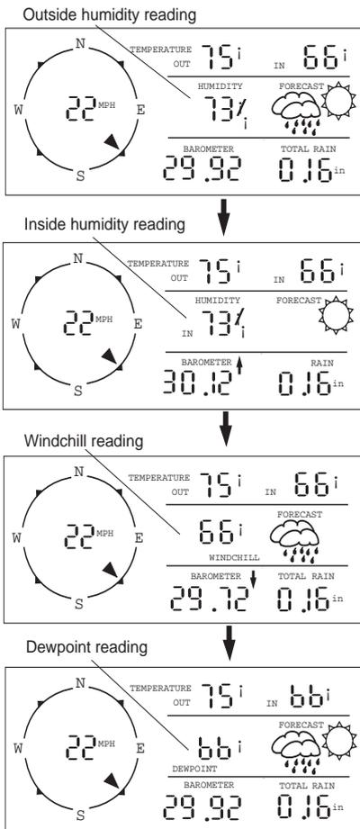
**Note:** At first power up, humidity and barometer readings, if available, do not display for up to one minute. The forecast displays in about 3 hours. (See page 21 for the update intervals thereafter.)
