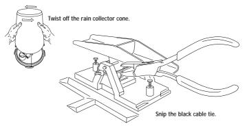
Do not re-attach the rain collector cone at this point; you will need to test the tipping bucket before you complete the installation.
