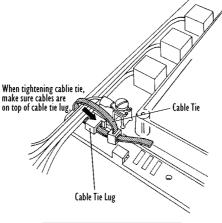
SECURING CABLES TO CABLE TIE LUG
