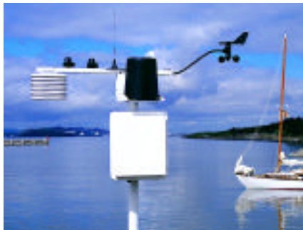
Health EnviroMonitor installation with cellular phone modem and omni antenna.
