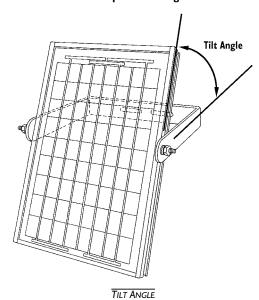
6. Tighten the hex screws on the mounting bracket until the solar panel is securely held at this angle.
