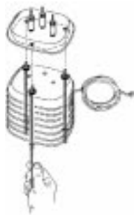
ATTACHING THE COVER PLATE ASSEMBLY TO SOLAR RADIATION SHIELD
