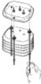
ATTACHING COVER PLATE TO SOLAR RADIATION SHIELD
