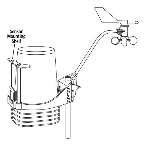
**Note:** This manual shows installation of the sensor mounting shelf before the two round solar sensors have been attached to it. If you like, the solar sensors can be mounted on the shelf before it is installed on the ISS. (Consult one of the sensor manuals for instructions.) **Final leveling of the sensors should be done after the ISS is mounted in its operating location.**
