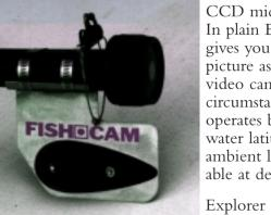
CCD micro camera system. In plain English, this system gives you about as good a picture as the best home video cameras, under most circumstances. This system operates best in the clearer water latitudes where ambient light is more available at depth.
