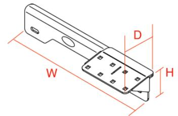
**Note:** Installing this base into the 2006 Dodge Charger/Magnum vehicles will compromise the vehicle air bag system, possibly endangering vehicle occupants. Seat bolts in 2006 vehicles are tied into the air bag sensor system. Loosening or removal of seat bolts in the 2006 vehicles will require recalibration by a certified Daimlyer-Chrysler service technician.
