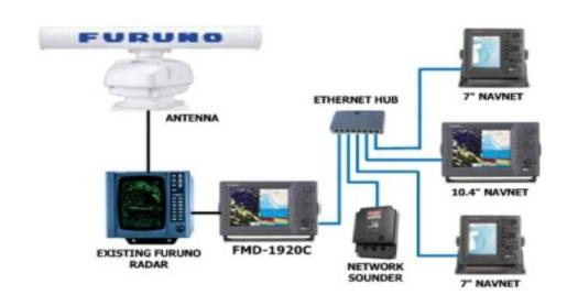
Note that changing the gain, STC or FTC on the master Furuno radars with Linear IF amplifiers (designated by a † symbol above) will affect the radar picture of the FMD-1920C. Additionally, Furuno radars with an \* require the optional buffer PCB, P/N 008-471-070. (This PCB is No longer available from Furuno USA)
