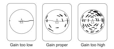
Examples of proper and improper gain
