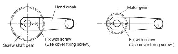
120 turns to move main shaft by 600 mm.
