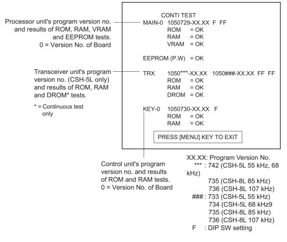
Continuous test (example: CSH-5L, 55 kHz transducer)
