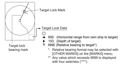
Target lock mark and target lock data
