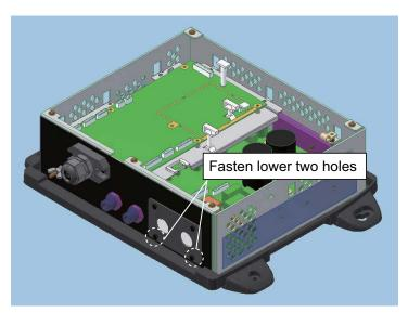
10. Use two screws to fasten the clamp removed at step 4.
