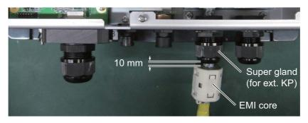
15. Attach the shield cover and close the outer cover.
