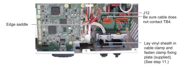
**Note:** For cable MPYC-2, tape the vinyl sheath of the cable (approx. 6 to 7 turns) where it lies in the cable clamp and fasten the cable clamp. The PH connector has two unused harnesses. Cut them at their base or wrap them with vinyl tape.
