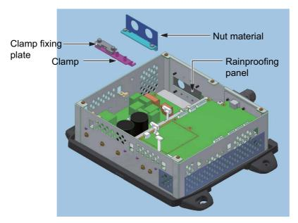
7. Using the two screws removed at step 5, fasten the upper two holes of the supplied rainproofing panel.
