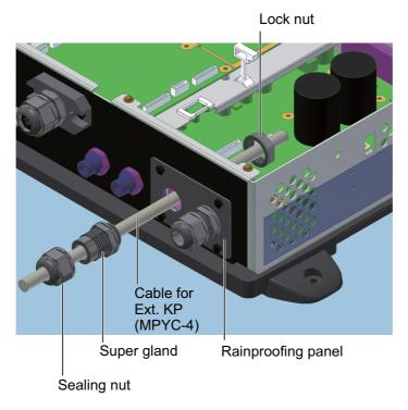
After passing the cable for the external KP, do as follows:
