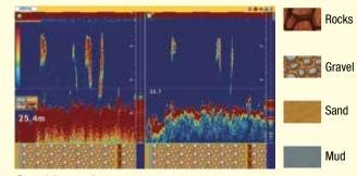
The standard graphic display mode shows the most probable bottom composition graphically as shown above.
