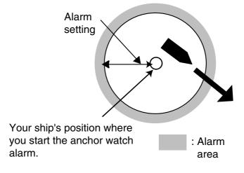
How the anchor watch alarm works
