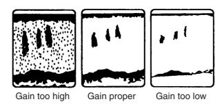
Examples of proper and improper gain
