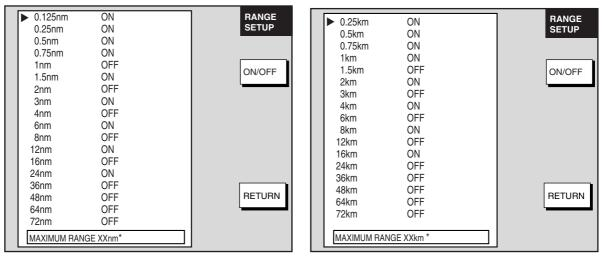
\* = Max. range depends on network radar used and is set on the network radar at installation.
