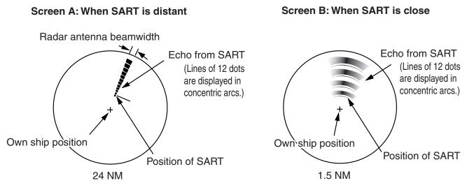
Appearance of SART signal on the radar display
