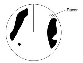
Appearance of racon signal on the radar display
