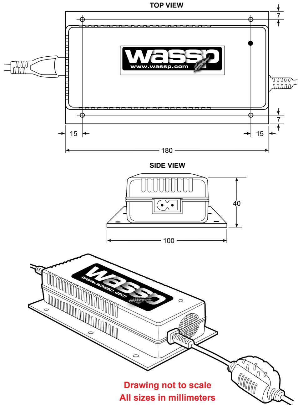
**Figure 10 – 24 V DC Power Supply Unit Mounting Bracket Outline and Dimensions**
