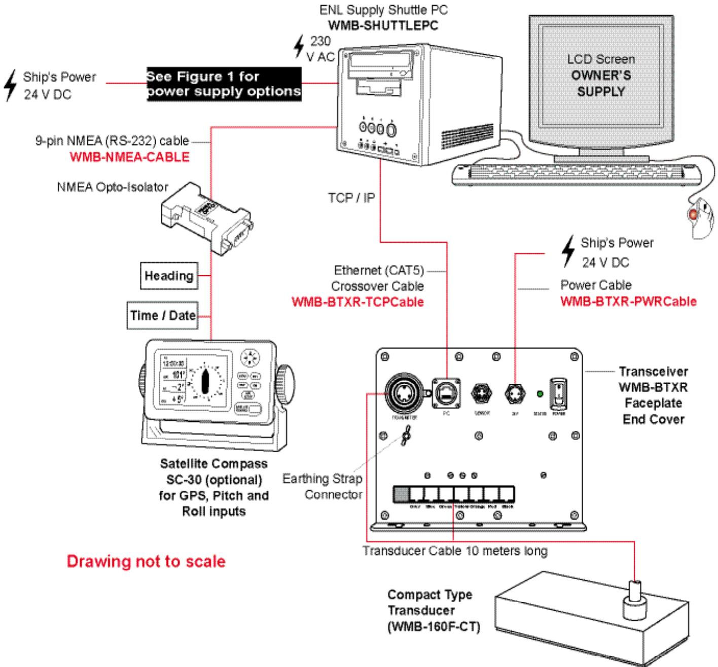
Figure 18 – WMB-160F Transceiver Interface Connections RJ-45 Type BTxR
