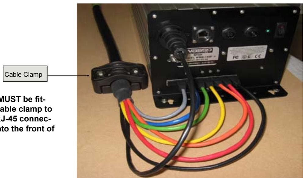
**Figure 16 – RJ45-type Transceiver Cable Clamp**
