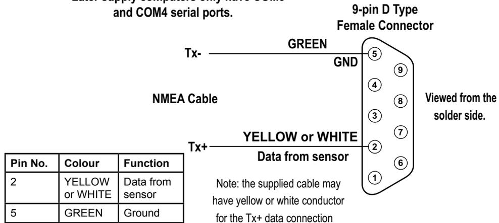
**Figure 20 – NMEA Connections and Pin out Diagram**
