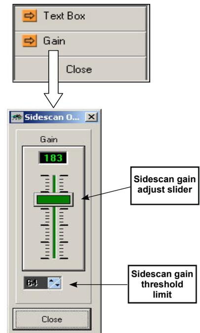
**Figure 38 – Sidescan Gain Setting Box**
