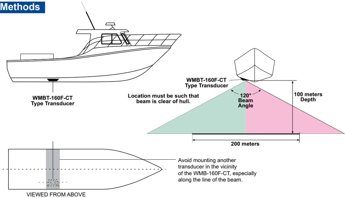
Figure 3 – Through-hull Compact Type Transducer Mounting
