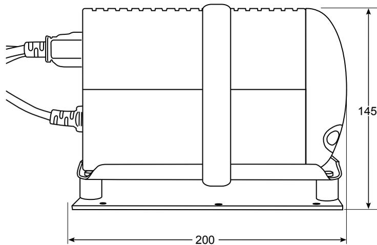
**Figure 9 – 230 V AC UPS Mounting Bracket Outline and Dimensions**
