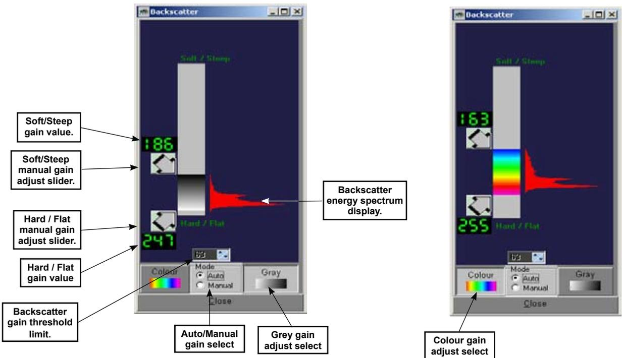
**Figure 40 – Grey and Colour Backscatter gain adjust boxes.**
