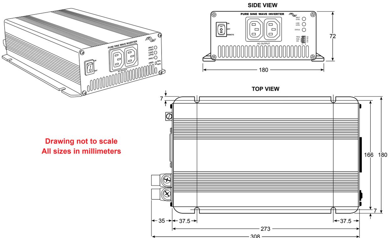
**Figure 11 – Inverter Mounting Bracket Outline and Dimensions**
