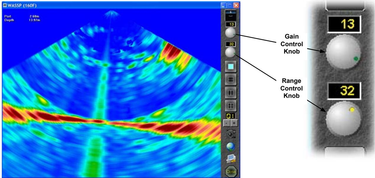
System with Significant Electrical Noise
