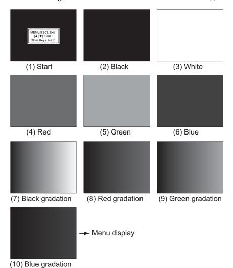
5. Control is returned to the menu after the blue gradation is shown. Press the **DISP** key to close the menu.
