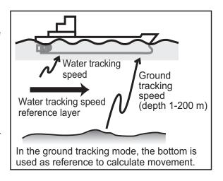
**Auto:** Automatically selects ground tracking mode or water tracking mode according to the depth. The water tracking mode is selected when the keel clearance is 200 m or more. (Actual working depth in the ground tracking mode depends on the bottom and water conditions, and the reflection properties for sonic pulses.)
