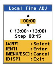
5. Use ▲, ▼ to set the time difference between local time and UTC time then press the ENT key.
