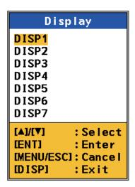
4. Select the display number (default display number for the graphic display is DISP5) where to show the speed graphic display then press the **ENT** key.
