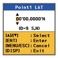
9. Use ▲ or ▼ to select the first digit of the latitude position then press the **ENT** key. Enter the remaining digits in the same method. (Use the **ENT** key to move the cursor right, and the **MENU/ESC** key to move the cursor left.)
