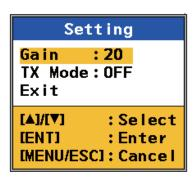
1) You can change the gain to see the echoes under different gain settings. Select [Gain] then press the **ENT** key.
