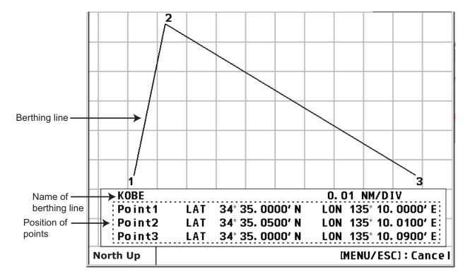
14. To save the line, press the **MENU/ESC** key to return to the [SET] dialog box (see the figure at the top of page 3-9). Press ▼ to show and select [Exit] then press the **ENT** key. (The berthing line is sent to all active sub display units when the **ENT** key is pressed.)
