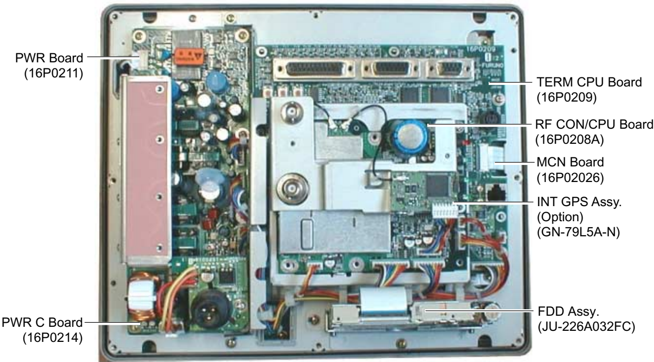
Terminal unit, inside view
