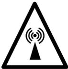
Do not approach the radome closer than 6 meters when it is transmitting.
