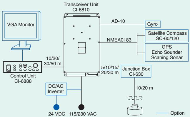
\*Display unit and control unit can be mounted separately with an optional cable
