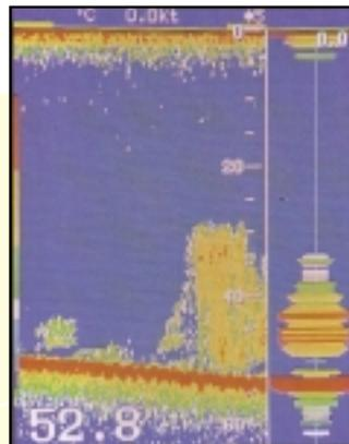
The A-Scope picture on the right 1/3 of the screen shows an instantaneous echo envelope at each ping, clearly showing echo differentials and positional relationship. This is useful for closer observation of target depth.
