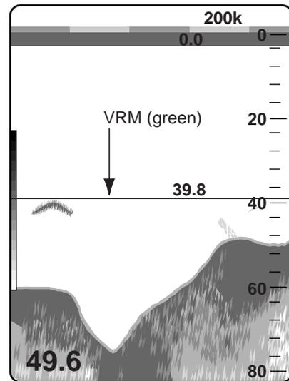
Figure 1-24 How to measure depth with the VRM
