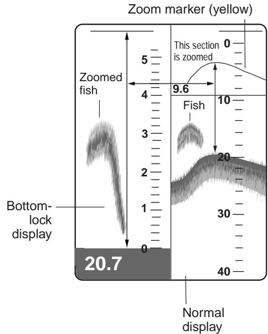
Figure 1-11 Bottom-lock display plus normal display
