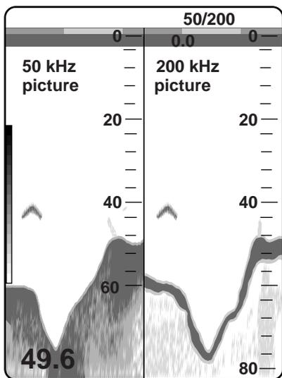
Figure 1-8 Dual-frequency display
