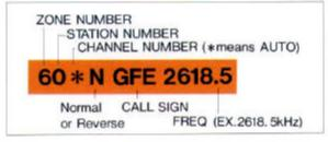
You do not have to know the frequencies of the fax stations. If you enter the ZONE and STATION numbers, the computerized receiver does everything else. To tune in the Bracknell station, for instance, hit the touchpads- $[CH][\blacktriangle$  to get 6 as ZONE][ $\blacktriangleright$  to move cursor][ $\bigstar$  to get 0 as STATION][ $\blacktriangleright$  to move cursor][ $\bigstar$  to get \* for automatic search][ENT].
