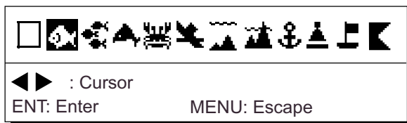
Figure 4-4 Screen for selecting waypoint mark shape
