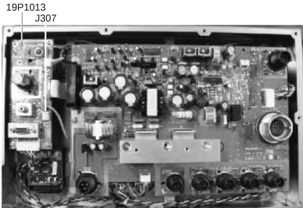
Processor unit (cover removed)
