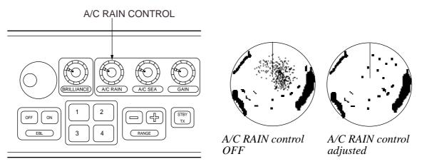
The A/C RAIN control adjusts the receiver sensitivity as the A/C SEA control does but rather in a longer time period (longer range). Clockwise rotation of this control increases the anticlutter effect.
