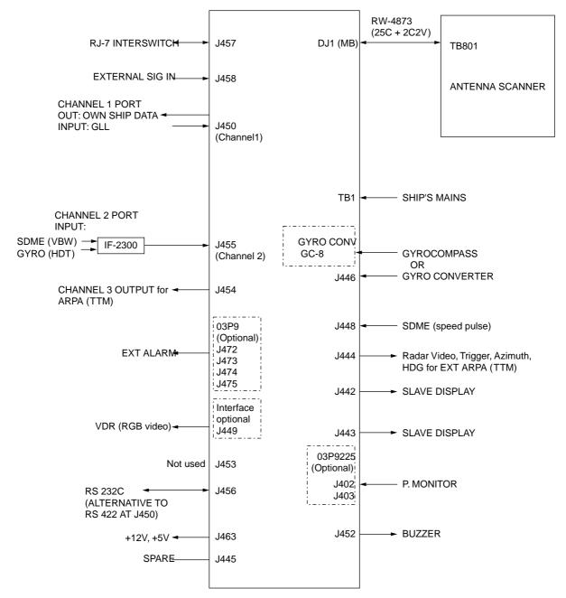
**Note:** The FR-2105/2105-B series radar does not process the IEC61162-2 data. Therefore, the system may only work as HSC radar by receiving data of gyrocompass data thru GC-8 or AD-100.
