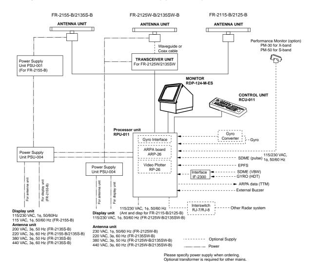
Note: The Display unit RDP-124 for FR-2105 series radar is separated into the Monitor RDP-124-M-ES, the Processor unit RPU-011 and the Control unit RCU-011 for FR-2105-B series radar.
