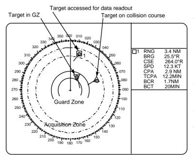
Target being accessed for data readout is marked  $\Box$ 1, 2,...etc.
