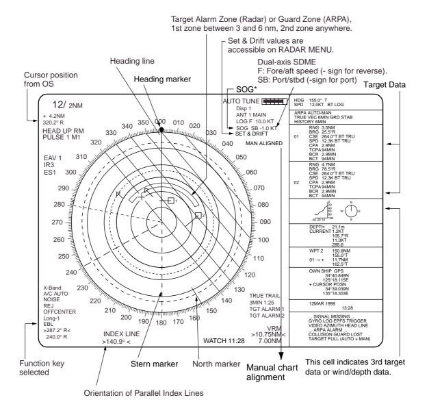
\*: With the serial speed inputs and SOG selection, if the type of data is changed from SOG to STW, the label SOG appears in red at the upper right corner on the screen.
