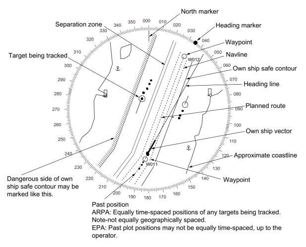
Concept of Radar map, Ground stabilized (Above excludes radar pictures. In reality, radar echoes are always displayed)
