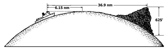
To calculate the distance to the horizon multiply the square root of the antenna height, in feet, by 1.23. To calculate the maximum range that you can detect a target with your radar add the square root of the antenna height to the square root of the target height and multiply by 1.23.
