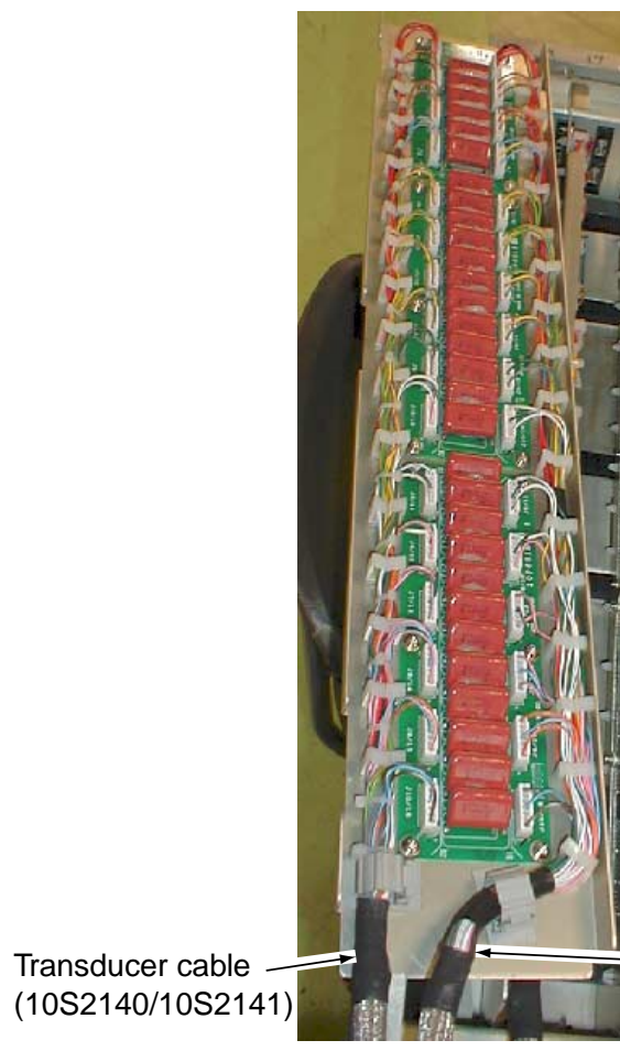
Junction box, cover removed, front view
