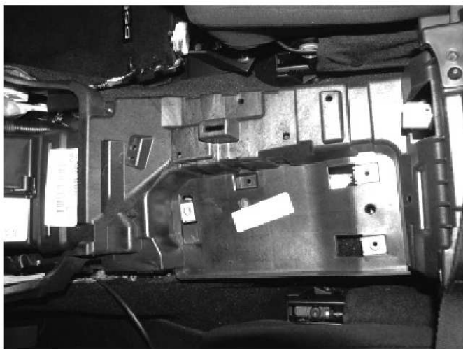
Fig 7 - Harness and Shifter Removed
