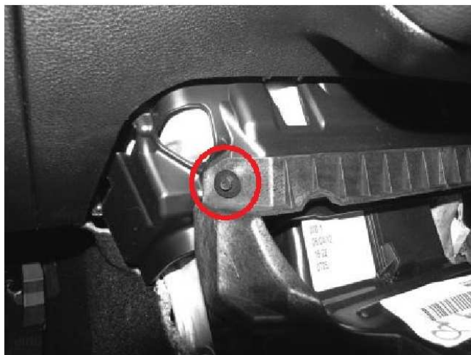
Fig 5 - Front Sub Structure Screws
