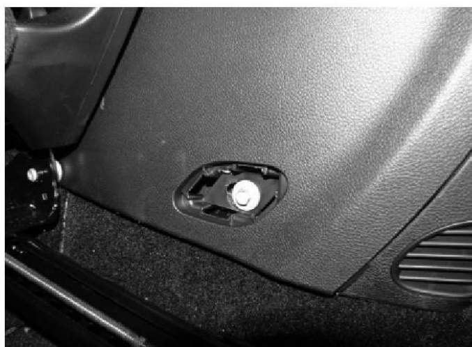
Fig 6 - Rear Mounting Bolts
