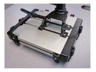
Attach Arm Assembly to the bottom side of computer Cradle or Dock with the (4) .25-20 x .50 long Socket Button Head Screws supplied with the Cradle or Dock.
