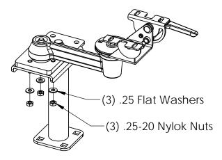
Remove the .25-20 nylok nuts and flat washers from the adapter plate. Place the adapter base on the upper pole assembly, inserting the threaded studs through the two radial slots. Place the washers and lock nuts on the studs and tighten. Unscrew the tilt knob to loosen clevis assembly and set the amount of tilt Lock in place by tightening knob.
