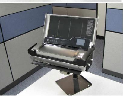
4. Insert printer into printer mount.
