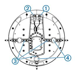
4 Press the cables into any of the guide grooves ③ on the bottom of the case, and secure them using a cable hold-down plate ④.
