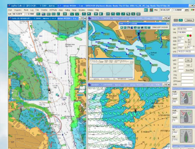
Multi function display with radar overlay and chart plotting
