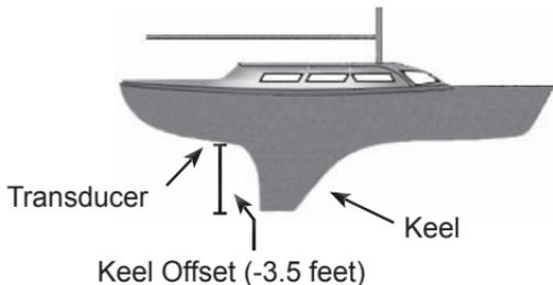
the distance from the transducer to the lowest part of the keel. If, for example, the keel is 3.5 feet below the transducer, it will be input as  $-3.5$  feet.
