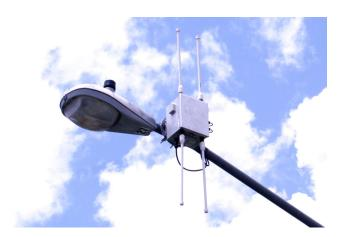
The Intelligent Access Point (IAP) acts as the transition point from the wireless network to the wired world. Each IAP offers a maximum burst data rate of up to 6 Mbps for voice, video and data communications. If greater network capacity is required, additional IAPs can be easily deployed – without the need for extensive RF or site planning. The location of IAPs is not critical due to the self-forming, self-healing and self-balancing nature of the MOTOMESH network.
