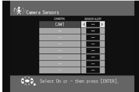
4. Use the navigator keys to select either [On] or [-] (off) for each camera's sensor, then press [ENTER].
