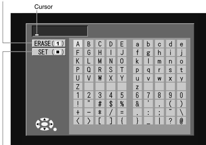
The text entered can be registered by pressing [STOP] or by selecting [SET] then pressing [ENTER]. The display will return to the previous screen.
