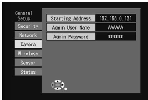
3. Move the mode switch on the BL-WV10A to Setup and turn the power on again.
