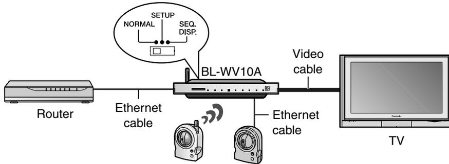
2. Set the mode switch on the back of the BL-WV10A to [NORMAL] and turn it on.
