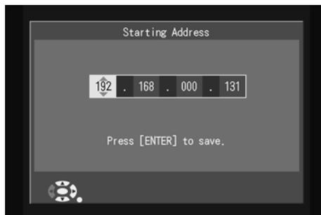
3. Enter the IP address for the camera and press [ENTER].
