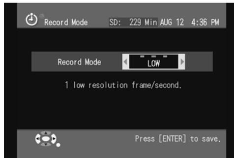
2. Using the left and right navigator keys, select the desired mode and press [ENTER].
