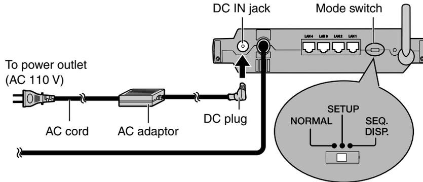
4. Confirm that the mode switch on the back of the BL-WV10A is set to [SETUP].
