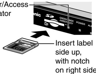
Insert label side up, with notch on right side
