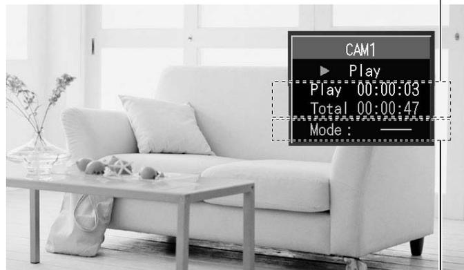
The recording mode (HIGH, LOW, LONG, or —) will be displayed. Movies recorded manually while monitoring the camera image will be recorded at the monitoring resolution and displayed as —.
