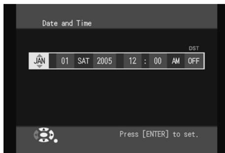
2. Use the left and right navigator keys to select the desired information, then press the top or bottom navigator keys to change the setting and press [ENTER].
