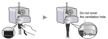
Attach the camera by screwing the threaded mount into the stand mounting hole.
