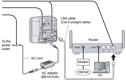
After the camera's indicator turns green, you may set up the camera. Continue by following the procedure described in the included Setup Guide.
