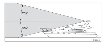
Mount the scanner so that the array rotates parallel to the waterline. The radar beam is approximately 25<sup>o</sup> wide in the vertical direction, giving good target detection when your boat pitches and rolls.
