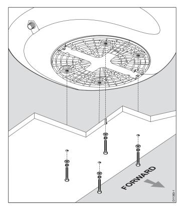
Securing the scanner to the mounting platform
