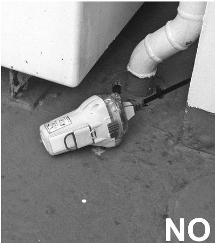
Fig. 5.3 – Incorrect siting of EPIRB
