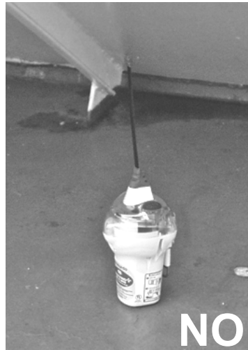
Fig. 5.3 – Incorrect siting of EPIRB
