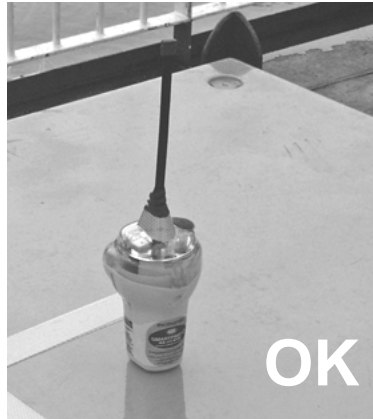
Fig. 5.2 – Correct siting of EPIRB
