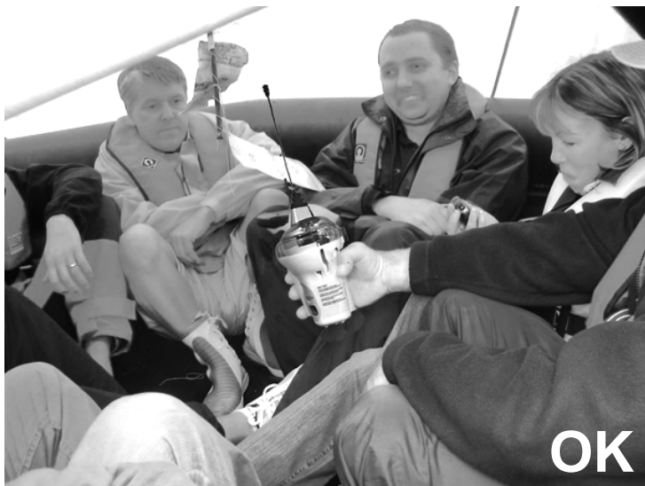
Fig. 5.4 – EPIRB in liferaft
