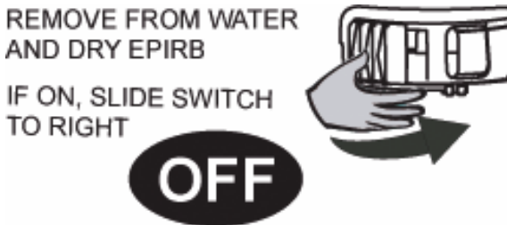
Fig. 5.9 – Deactivation of EPIRB
