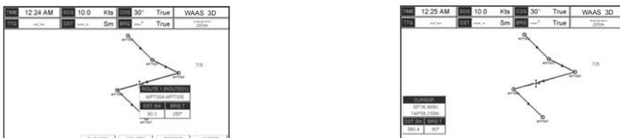
Figure 9.5 - Inserting Waypoint procedure (1)
