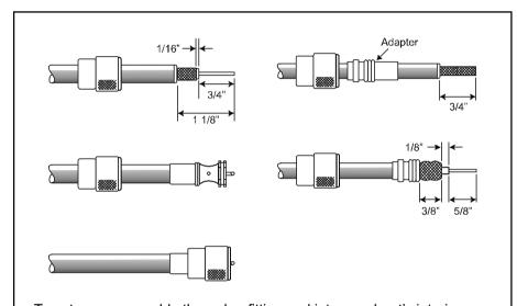
To get your coax cable through a fitting and into your boat's interior, you may have to cut off the end plug and reattach it later. You can do this if you follow the directions that are supplied with the connector. Be sure to make good soldered connections.
