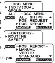
Press the \_\_\_ / \_\_ keys to scroll through numbers, 0-9. To enter the desired number and move one space to the right, press the \_\_\_ key. Repeat this procedure until all nine spaces of the MMSI number which you want to contact are entered.
