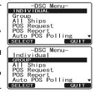
municate on, then press the SELECT soft key. If the channel you want is not shown, press the MANUAL soft key, then press the Alexander to select the operating channel you want to communicate on, then press the SELECT soft key.
