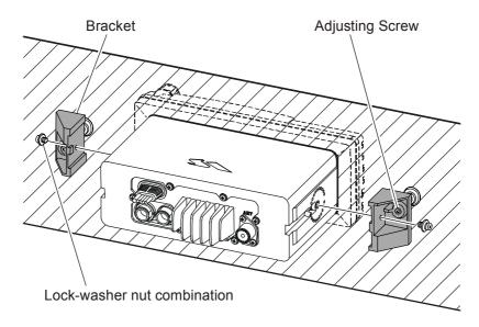
Figure 2. MMB-84 Flush Mount Installation
