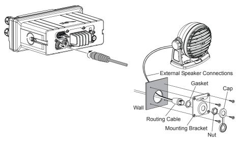
Figure 3. Enhanced RAM+ MIC Installation
