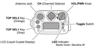
Blinking Green: Busy Channel (or SQL off) Steady Red: Transmission inProgress Blinking Red: Battery voltage is low
