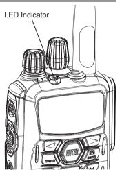
radio is transmitting and blinks green rapidly when the radio is receiving a privacy-enabled call.
